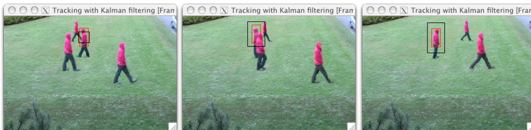
Figure IV.1: Search box resizing when loosing track of the target
